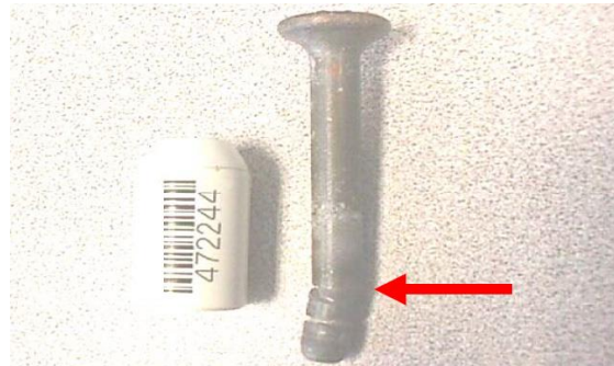
Seal stem is bent and does not lock properly.
