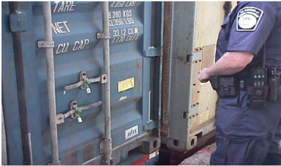
Check for excessive damage or alteration of seal.
