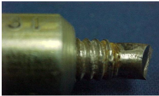
Twisted counter-clockwise and came off.
