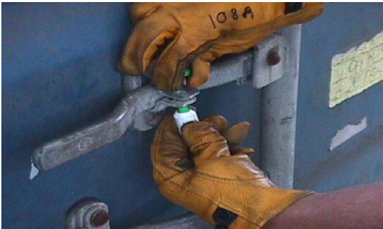
Seal must not loosen or come off when twisted and turned.
