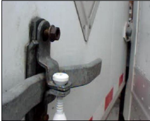
Loose container lock appearing to be locked with a seal.
