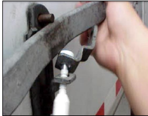
Container lock is manipulated for easy opening.
